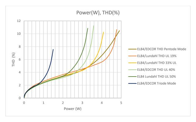
For a more detailed analyses, THD and the components k2/3 are then measured in the respective operating mode.
