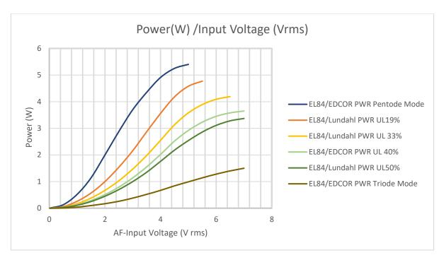
Subsequently those operation modes are evaluated in respect to total harmonic distortion (THD) (K2 - K4). As expected, the UL-traces are moving gradually from the pentode-trace towards the triode trace as the percentage of UL tab increases. The available power, limited by the onset of clipping, is continuously decreasing. Due to its low gain, the triode operation provides the least power output. According to this diagram, the pentode operation could be suspected to be superior to all others.
